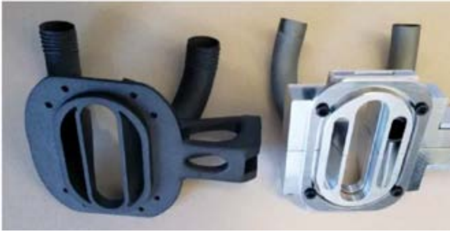
Figure 7: A 3D printed part used by HP. Compared to the machined and assembled part on the right, the 3D printed part reduced mass from 575 grams to 53 grams, reduced part count from 5 to 1, lowered cost by 91%, and reduced lead time by 91%. 14
